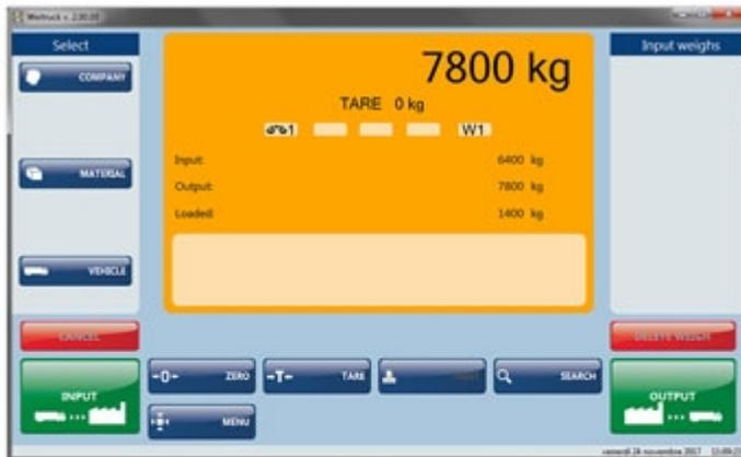
Software for a PC which allows to completely manage a weighbridge system, combinable to the DFW, DGT and 3590 series' weight indicators. Besides the complete management of the connected scale, the programme offers a simple and intuitive operator interface, databases for the storage of the customer, material, and vehicle data, management of the totals and programmable printouts.
